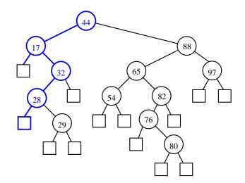
• An unsuccessful search traverses a path starting at the root and ending at an external node
