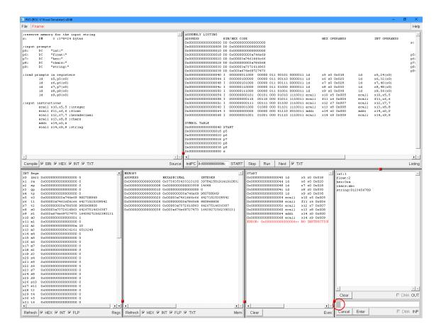
An active input is indicated by a blinking rectangle (its color will be altering from gray to red and vise versa.) The rectangle is denoted by a red circle in the screen snapshot above.
