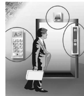
Figure 1: A Miconic-10™ keypad allows passengers to enter their destination before they enter the elevator. A display informs the passenger about the elevator that will offer the most suitable transport.
