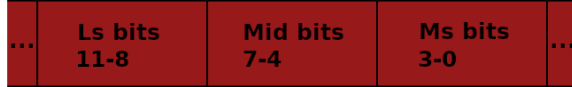
Figure 2. Address storing convention for virtual address registers with least (resp. most) significant nibble first (res. last).
