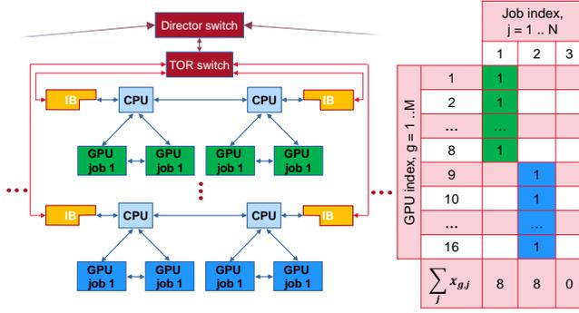
**Figure 2: (Left)** A rack is shown with its Top of Rack Switch (TRS), and two of its machines. The vertical ellipsis mean that there exists additional machines. Horizontal ellipsis on either side mean there may exist additional racks. The dark red arrows pointing to the DS indicate connections from two additional TRS's on either side. **(Right)** Example assignment of GPUs 1 to 8 for job 1 and GPUs 9 to 16 for job 2.
