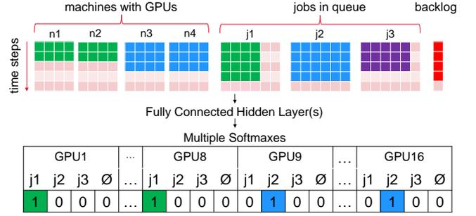
**Figure 1: The architecture of the NN function approximator. Above there are three jobs in the queue. The first two are running, and the third is waiting. This assignment is not optimal but possible, depending on the level of training.**
