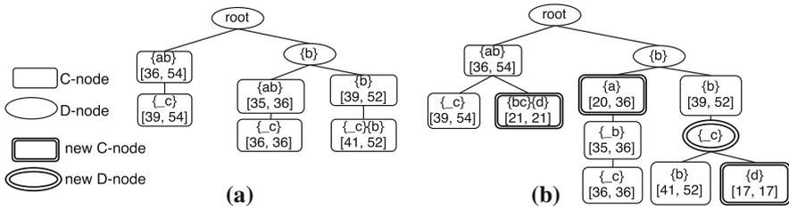
**Fig. 3** **a** An example of MAS-Tree for  $B_1$  in Fig. 1. Note that an underscore in a node name  $\{\_c\}$  means that the last itemset in the pattern of its parent, such as  $\{ab\}$ , belongs to the first itemset of the pattern of this node. That is  $\{ab\}$  and  $\{\_c\}$  forms  $\{abc\}$ , **b** MAS-Tree after inserting three patterns:  $\{\{ab\}\{bc\}\{d\}\}$ ,  $\{\{b\}\{a\}\}$  and  $\{\{b\}\{bc\}\{d\}\}$
