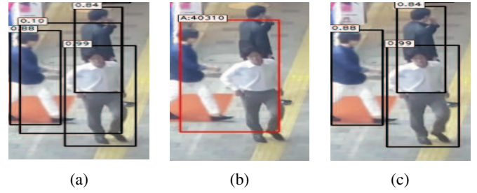
Fig. 3: Part of the Frame-206 taken from the MOT17-04 video sequence. (a) Four bounding boxes detected by KDNT detector, (b) The outlier (wrong) bounding box has been correctly isolated by the proposed post-processing algorithm (Step 1 in Section II-A), (c) Three true positive bounding boxes are correctly retained after applying the proposed method. The complete video is available at https://youtu.be/CytR_WFF5ys
