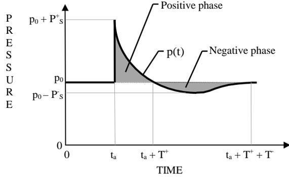
Figure 2-1. Pressure-time curve of an ideal blast
