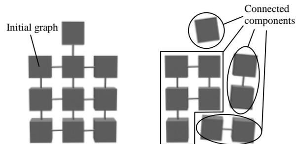
Figure 3-2. Graph representation of the connected voxel model
