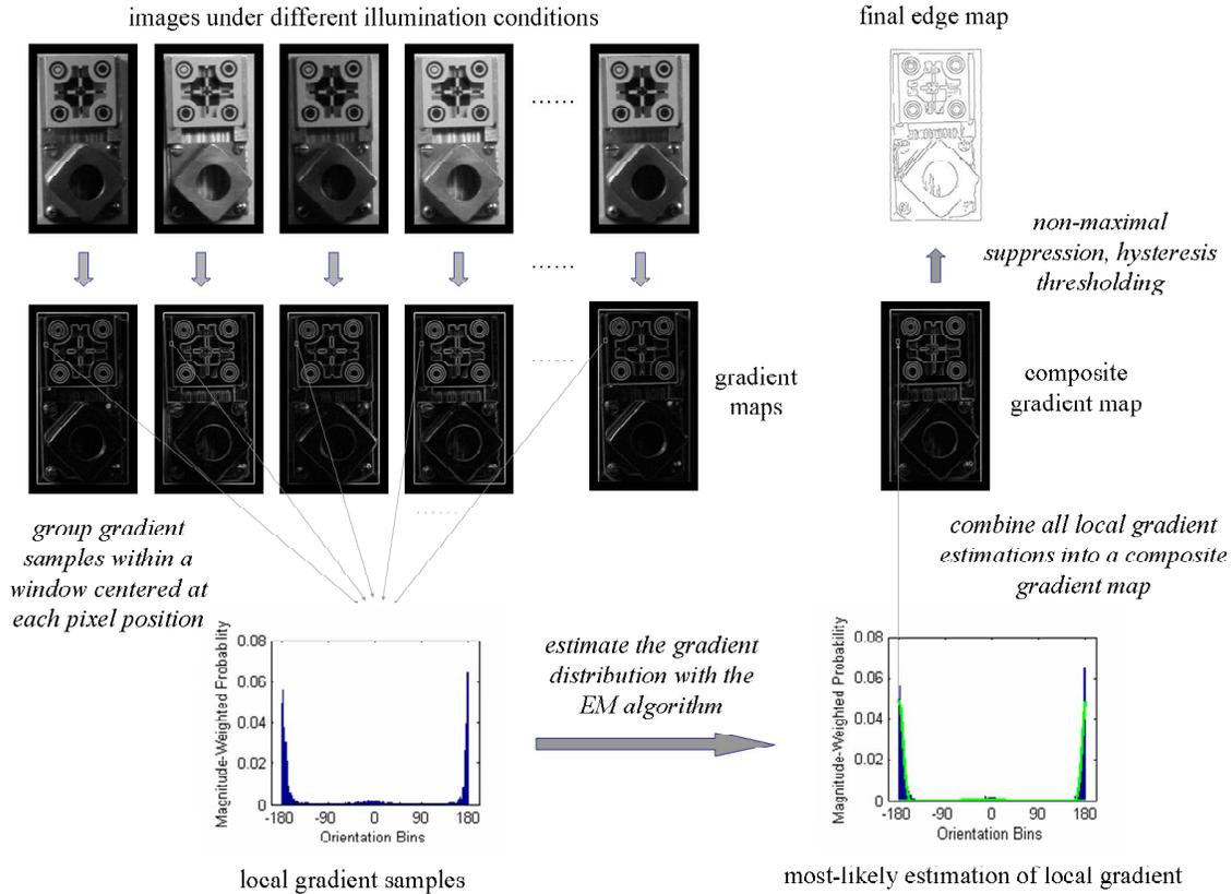
**Figure 4. Outline of the multi-channel edge detection algorithm.**
