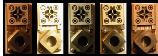
**Figure 2. Views of the Dextrous Handling Target and Micro Fixture under various illumination conditions. Pose estimates computed from these images are used to capture the fixture autonomously.**
