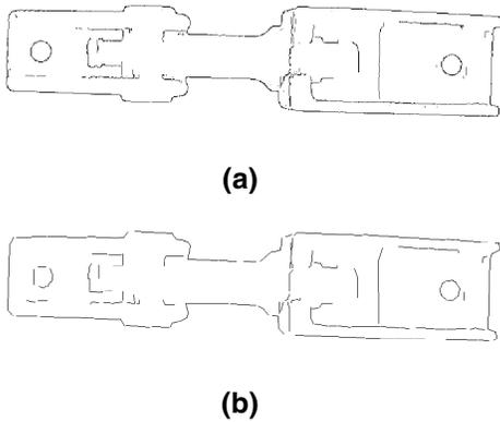
**Figure 5. (a) Multi-channel edge map of a Hubble Space Telescope Latch. (b) Its polyline approximation.**
