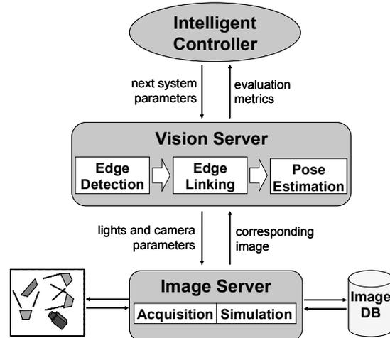
Figure 3. The Lights and Camera system architecture.
