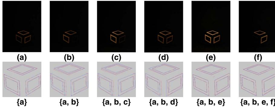
**Figure 7. The images acquired (top row) and the model matching result and edges recovered (bottom row) during the six iterations of the sample run. Images (a), (b), (e) and (f) were selected by the Controller for the final pose estimation.**
