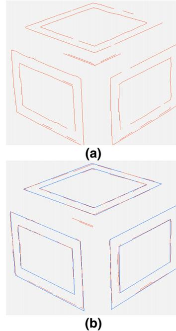
**Figure 6. (a) Multi-channel polyline data for a textured cube. (b) The resulting model match data overlaid on (a).**
