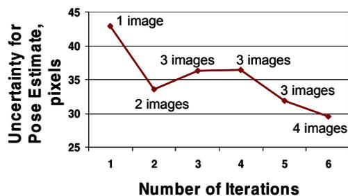
**Figure 8. Sample run of the “Lights and Camera” system. For each iteration of the control loop, the number of images used in processing is given.**
