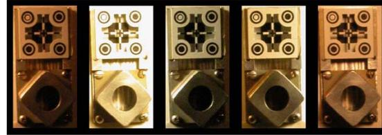
**Figure 2. Views of the Dexterous Handling Target and Micro Fixture under various illumination conditions. Pose estimates computed from these images are used to capture the fixture autonomously.**
